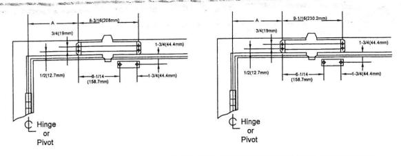
Left hand door shown Right hand door shown Dimensions are in inches Do not scale drawing
