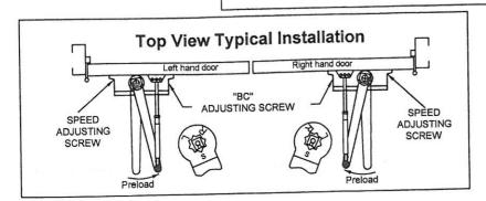
TDC 50 SERIES (With Back Check) Installation Instructions for TOP JAMB (PUSH SIDE) Mounting THIS TEMPLATE COVERS REGULAR ARM INSTALLATIONS TO 180° OPENING.
