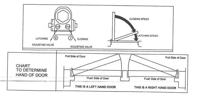
TDC 50 SERIES (With Back Check) Installation Instructions for REGULAR ARM (PULL SIDE) Mounting THIS TEMPLATE COVERS REGULAR ARM INSTALLATIONS TO 180° OPENING.
