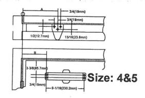
Left hand door shown Right hand door shown Dimensions are in inches Do not scale drawing
