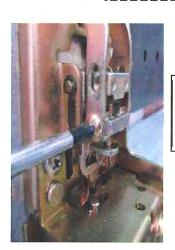
Secure the connecting bar to the slider with two side screws.
