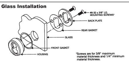
**Note:** Material thickness can be changed by using an "0" ring or changing the screw length.
