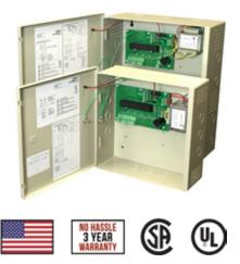
**PS202/202B** – 110-120VAC input power supplies that deliver (2) amps @ 24VDC to (2) PTC fused outputs. (2) solid-state input triggers, protects system relays from shorts, grounds and surges. Its linear design makes it a perfect match for electric locks, motor driven exit devices, electric strikes, and mag locks.
